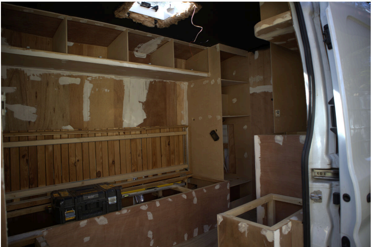
All filled and sanded — ready for the final finish
