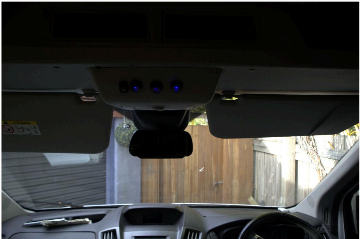
Cockpit control switches — hot water, water pump, and grey water release all accessible from the driver's seat
