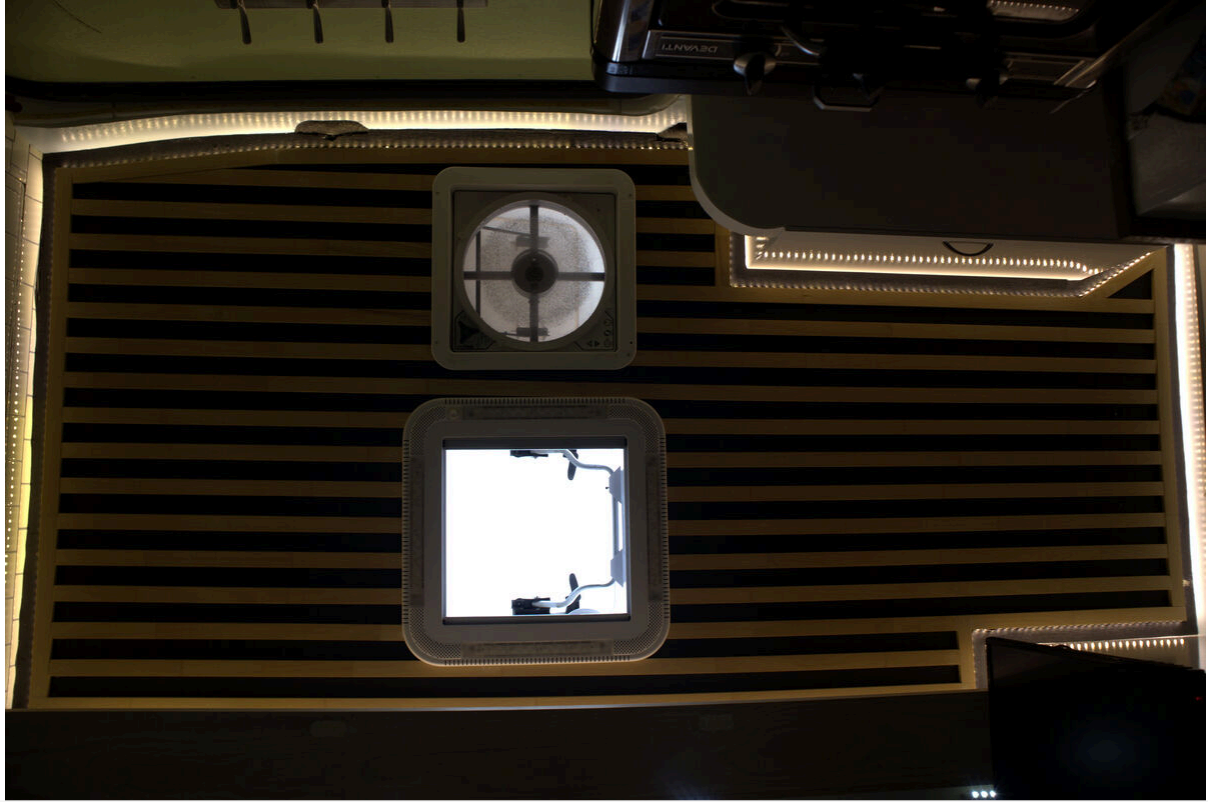
The finished roof — pine strips with warm white LED lighting around the edges
