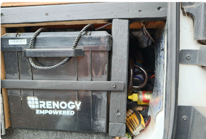
Lithium battery upgrade and solar controller wiring
