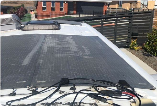
Left: Initial flexible panels for stealth. Right: Upgraded rigid glass panels on Sikaflex-bonded brackets
