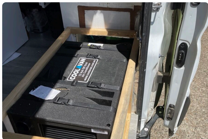
The air conditioning upgrade — looked good but drew 60 amps constant
